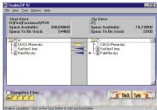
Compression uses the PKZip algorithm so you can share backed-up files with almost anyone
